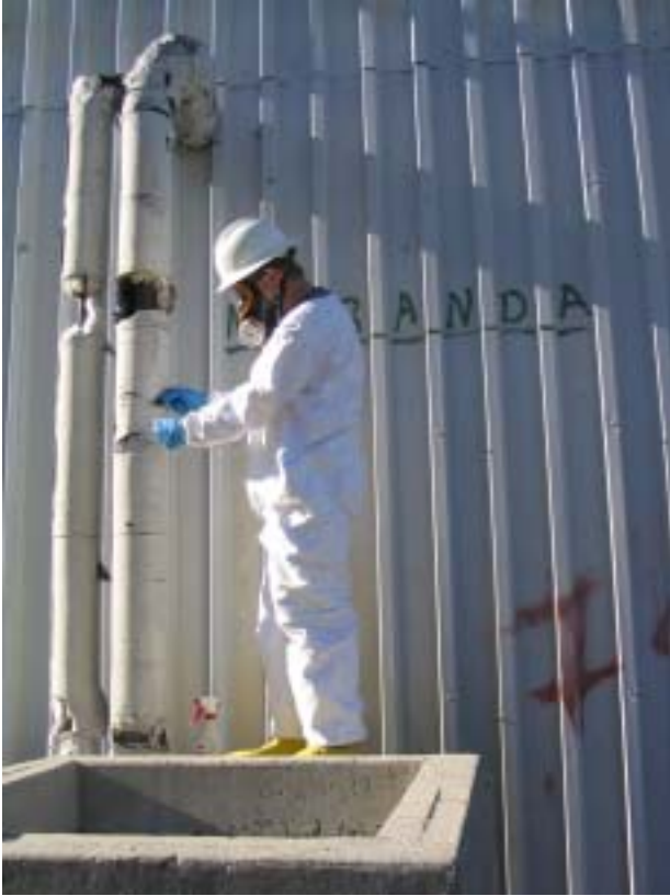
Photograph 13. START-2 collects bulk samples for asbestos analysis.
