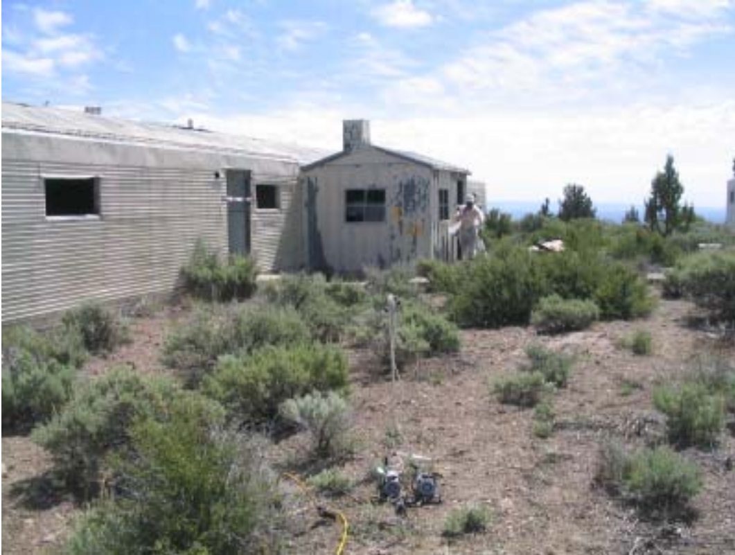
Photograph 31. Air sampling pumps near area of asbestos abatement.
