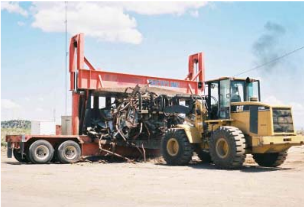
Photograph 38. Steel recycler consolidates scrap steel with metal crusher.
