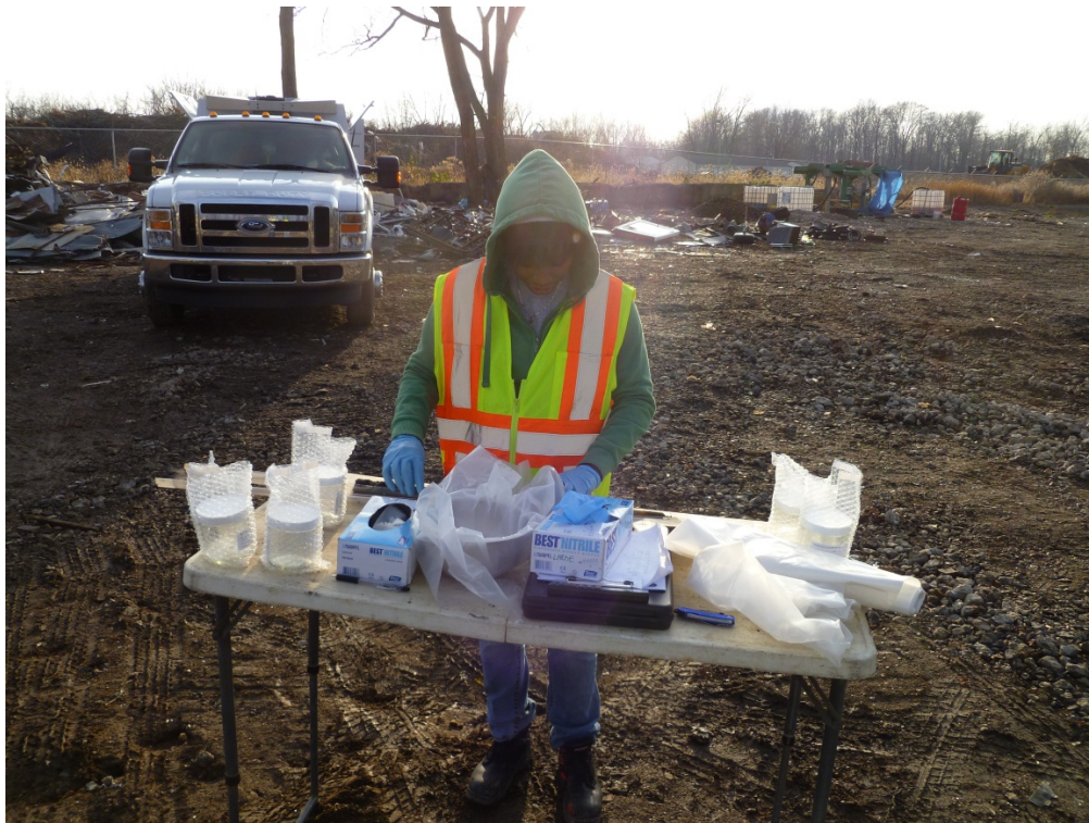
Photograph No.: 8 Photographer: Santino Nardulli Orientation: Looking West TDD Number: TO-01-12-10-1012 Contract: EP-S5-10-10, OTIE Date: 12/03/12 Site Name & Location: Dixon Road Site, Kokomo, Howard County, Indiana Subject: START preparing soil boring sample for analytical analysis.
