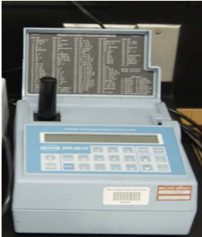
Figure 4-12. HACH® DR/2010 spectrophotometer.
