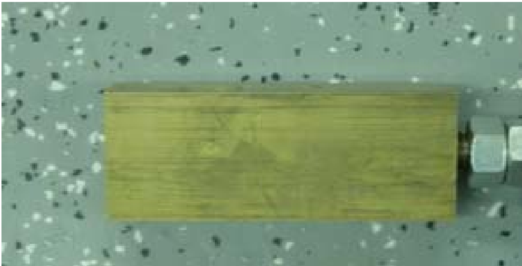
Figure 4-5. Close up view of compaction hammer head.
