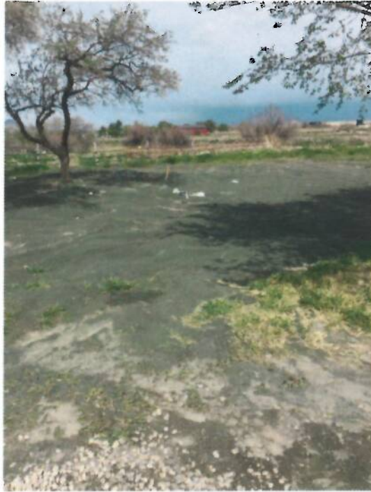
Photo 1: View of contaminated soil on the property. The spent sand blasting material can be seen as the green discoloration.
