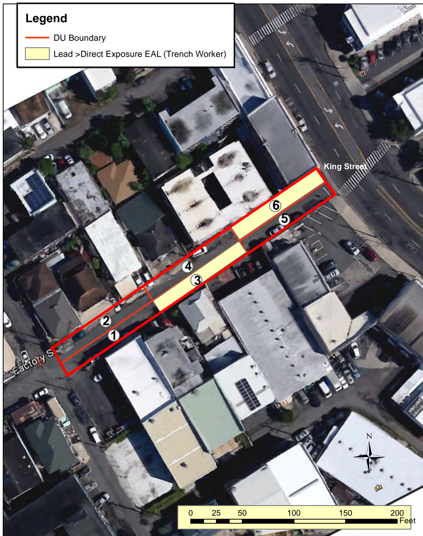
Figure 6b: DUs of 2017 Site Assessment with lead > 800 mg/kg at 0.5 to 1 ft bgs
