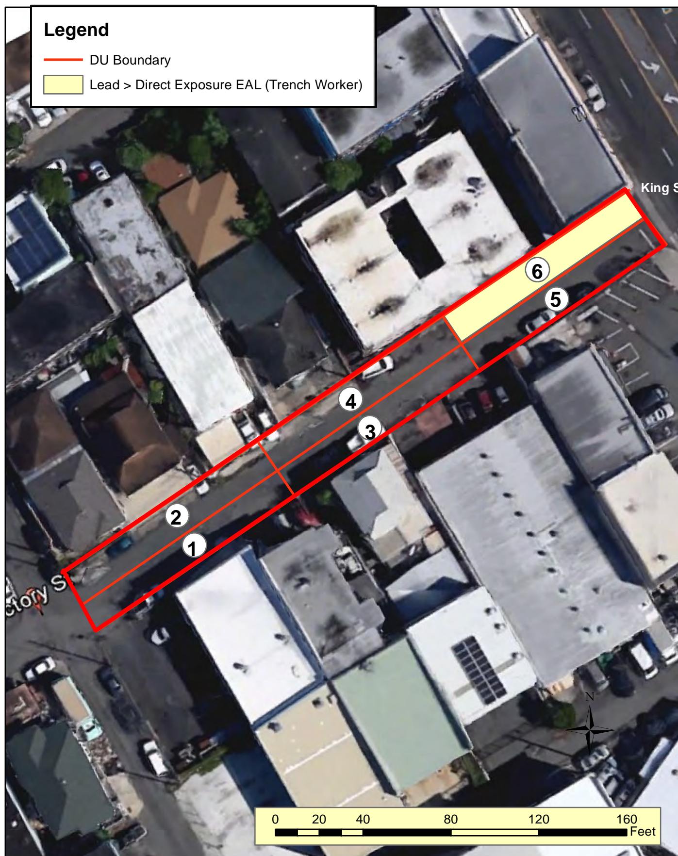
Figure 6c: DUs of 2017 Site Assessment with lead > 800 mg/kg at 4 to 5 ft bgs
