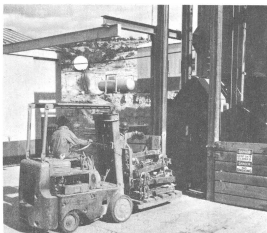
FIGURE 24. - Lifting Pallet of Props on Cage.
