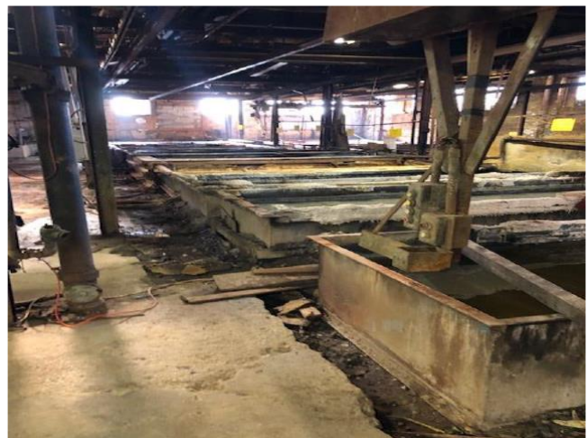
Picture of plating line with cyanide, caustic and acid vats.
