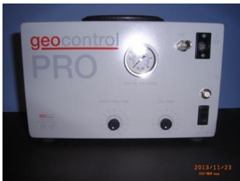
Air Activated Bladder Pump
