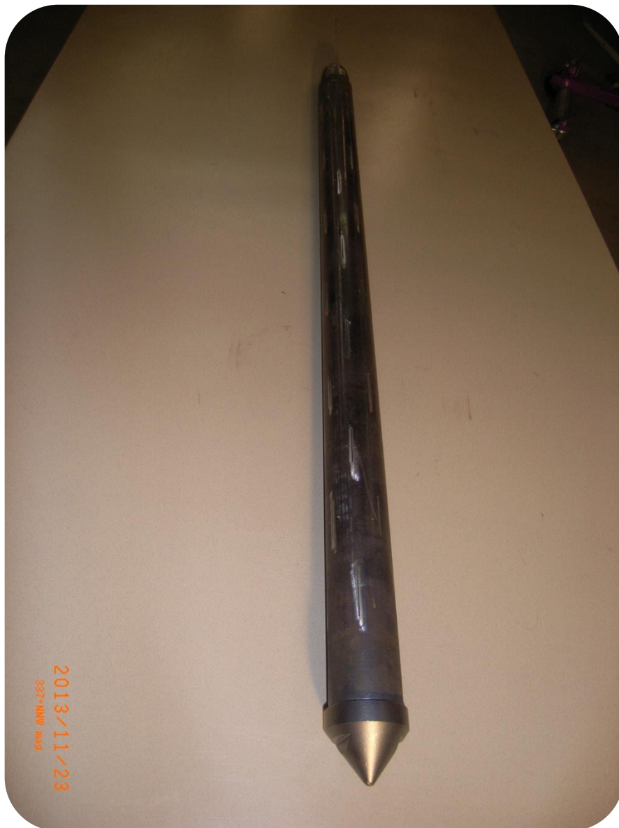
Mill Slot Probe Rod for GW Sampling
