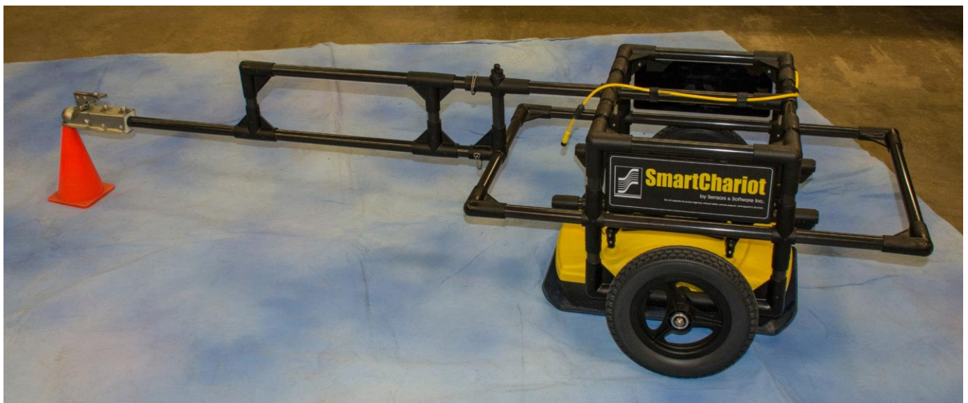
GPR configured to be towed by ATV for large sites.
